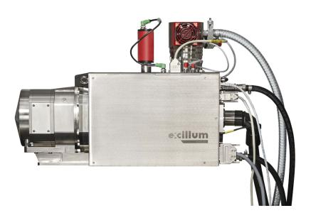
The Excillum NanoTube N3 enables industry-leading resolution and stability in geometric-magnification X-ray imaging systems with no need for manual tuning. It is based on advanced electron optics and the latest tungsten-diamond transmission target technology. Automatic e-beam focusing and astigmatism correction ensures that the smallest possible, truly round spot is achieved every time, every day.
