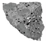
A 3D rendering of the phasecontrast Nano-CT of a basalt sample, revealing the different phases, elements and structures help geologists to further understand this sample. Voxel sampling 350 nm.
