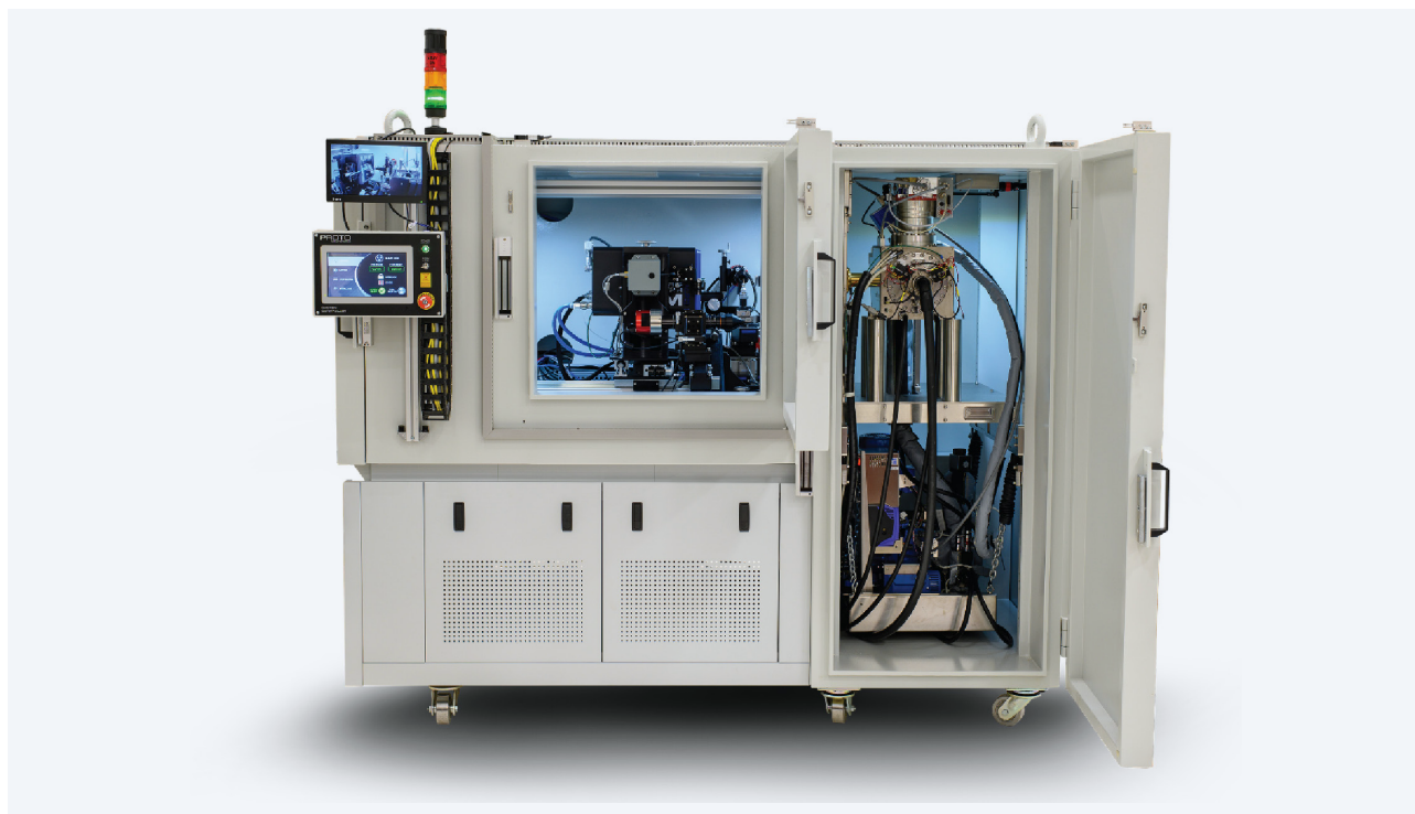
Figure 6: An example of a High Pressure X-ray instrument from PROTO combining an EIGER2 CdTe 4M detector with a In MetalJet source.
