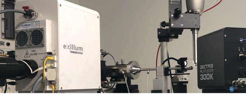
66 If the data collection is not successful with the conventional X-ray diffractometer, I run the test again with the high intensity MetalJet and PILATUS combination to get much better quality data."
