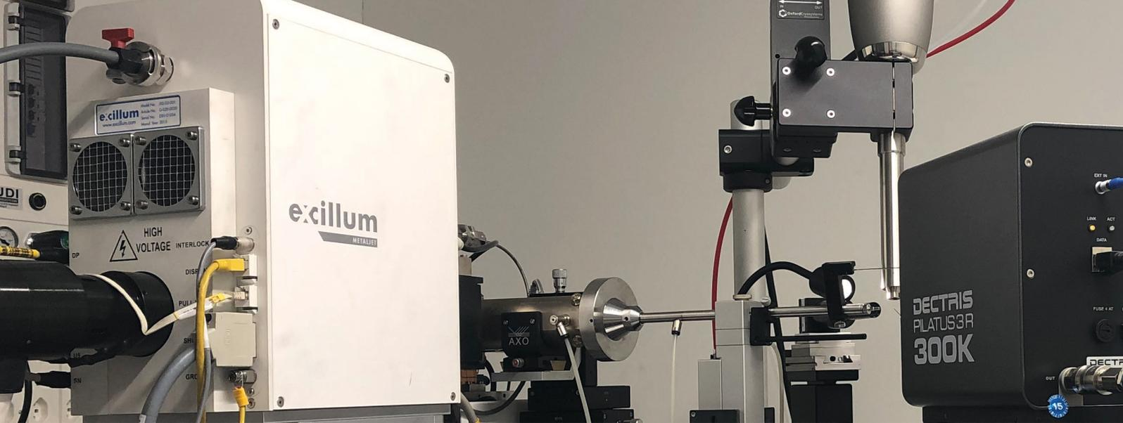
“If the data collection is not successful with the conventional X-ray diffractometer, I run the test again with the high intensity MetalJet and PILATUS combination to get much better quality data.”
