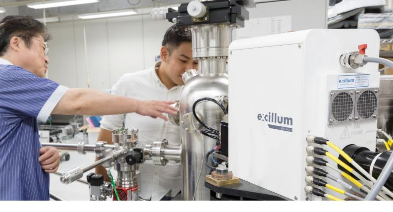
resolution better than 0.6 eV and a focus on the sample of 50  $\mu$ m. This, together with an electron spectrometer and UHV sample environment, forms the laboratory HAXPES system, called HAXPES-Lab.
