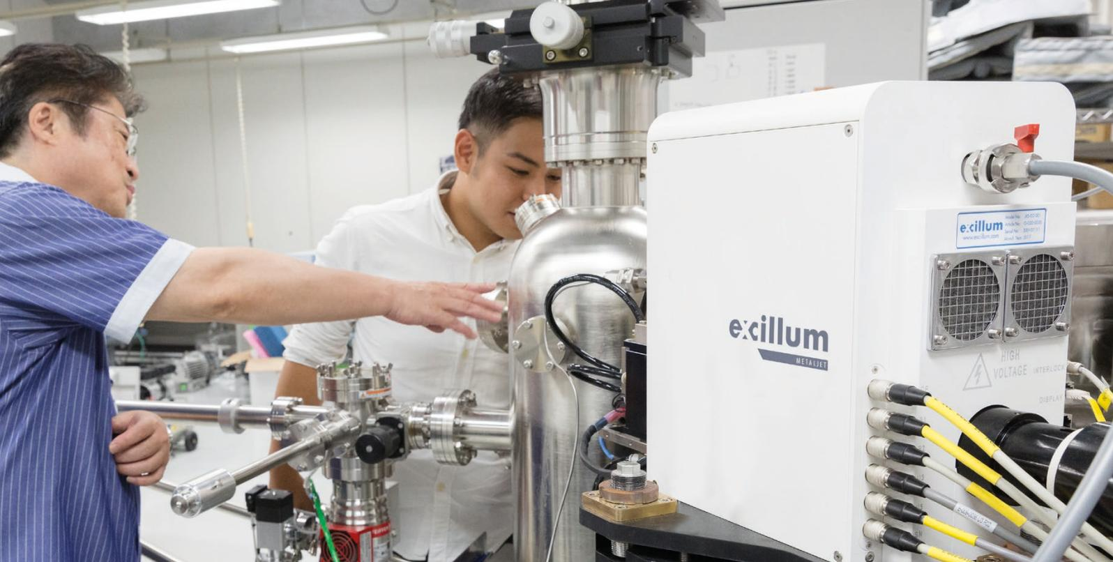
resolution better than 0.6 eV and a focus on the sample of 50  $\mu\text{m}$ . This, together with an electron spectrometer and UHV sample environment, forms the laboratory HAXPES system, called HAXPES-Lab.
