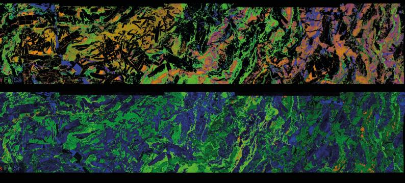
12 M pixel RGB false-color images of a drill core segment (236 x 46 mm2) from the Abra lead-silvercopper-gold deposit in Western Australia (7867 x 1533 pixels, each 30 µm at 5.3 ms dwell time) acquired using Maia Mapper and an Excillum MetalJet D2+ at 200 W and 70 kV into an effective 20 µm source size.
