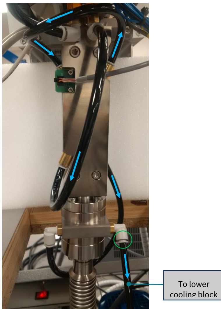
Figure 4-12. Upper cooling block with water hoses connected and flow direction indicated with blue arrows.
