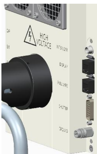
Figure 4-19. X-ray head from behind (right side) showing the connectors for the safety system interface.
