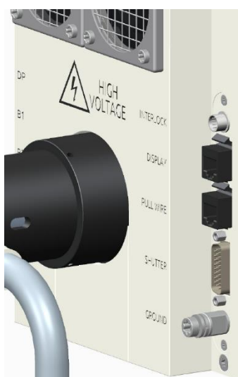
Figure 4-23. X-ray head from behind (right side) showing the connectors for the safety system interface.
