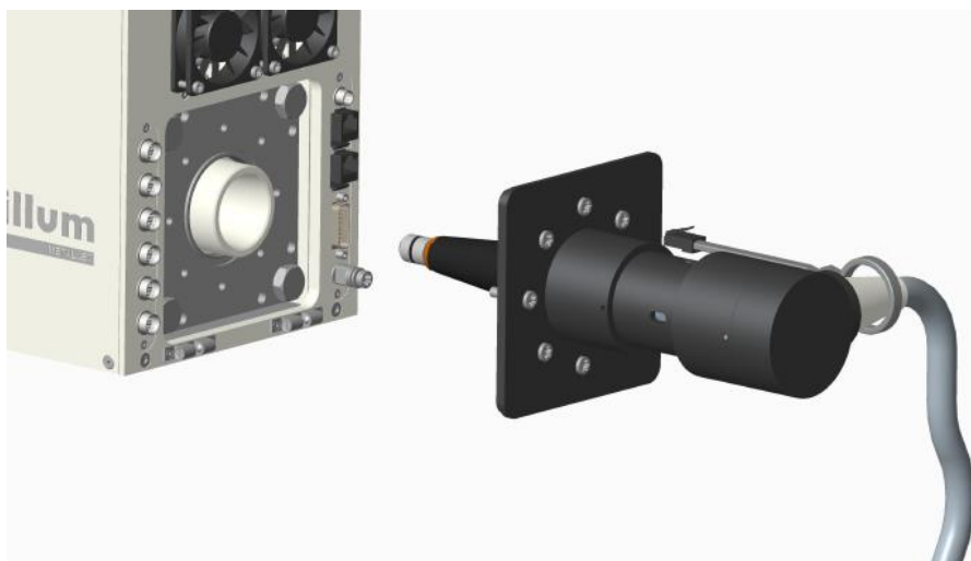
Figure 4-18. Connect the tapered end of the high voltage cable to the electron gun according to the instructions above.
