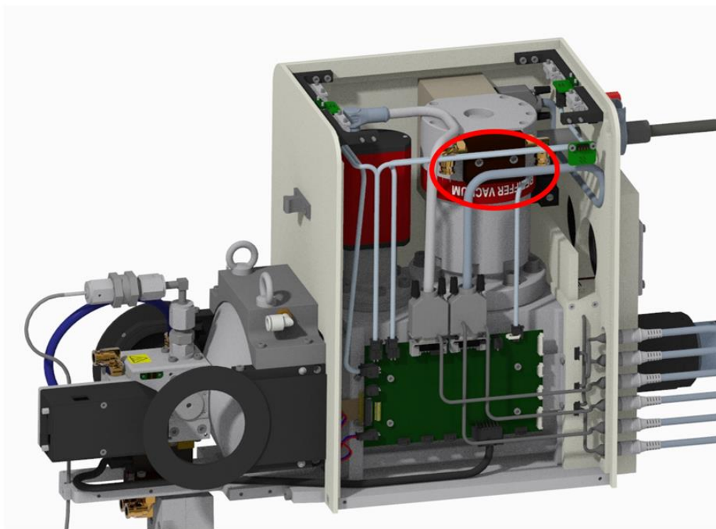
Figure 4-11. X-ray head with right hand cover removed. Turbo pump cooling block circled in red.
