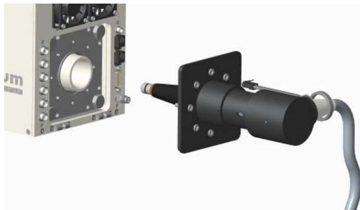
Figure 2-1. Always ensure complete discharge of the high-voltage cable when removing it from the source by letting the circled metal connectors touch ground.
