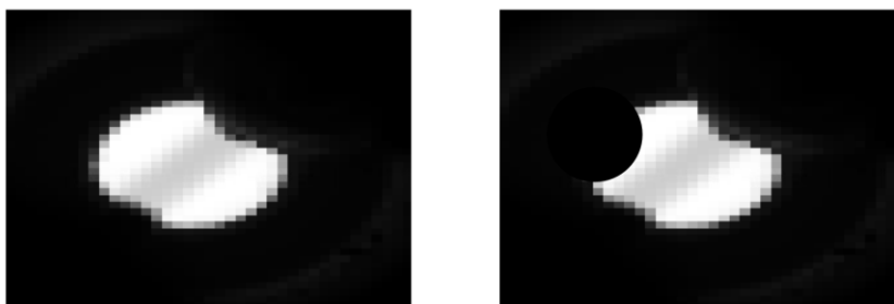
Figure 5-6. Align of clean (left) and contaminated (right) electron-beam dump aperture.
