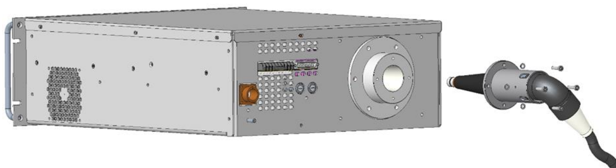
Figure 4-24. Connect the ribbed contact of the high voltage cable to the rear of the X-ray high-voltage controller unit.
