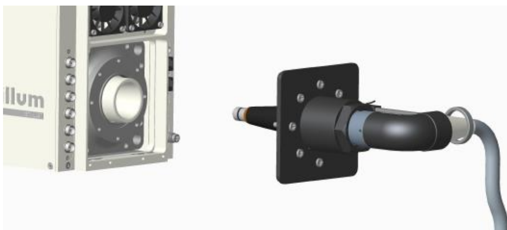
Figure 4-22. Connect the tapered end of the high voltage cable to the electron gun according to the instructions above.
