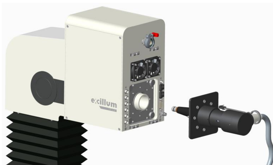
Figure 4-31. Allow for enough clearance to remove the high voltage cable and high voltage flange during cathode replacement.
